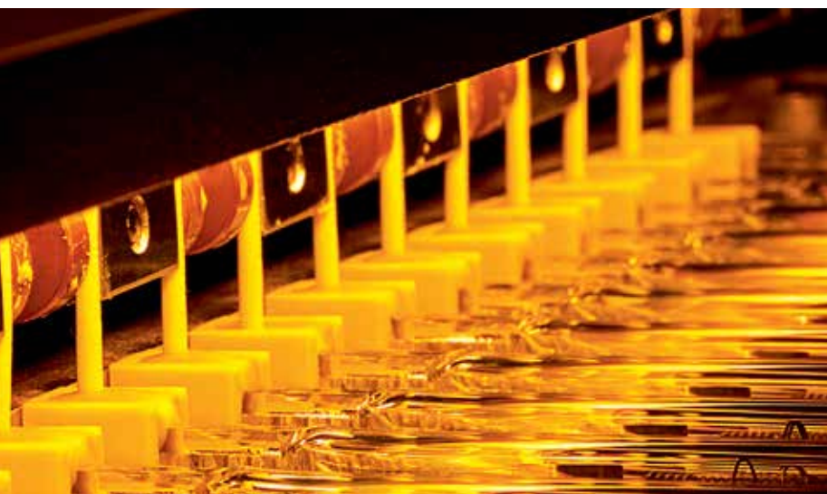
Infrared drying of ceramic bases and connection to the quartz lamp tube
